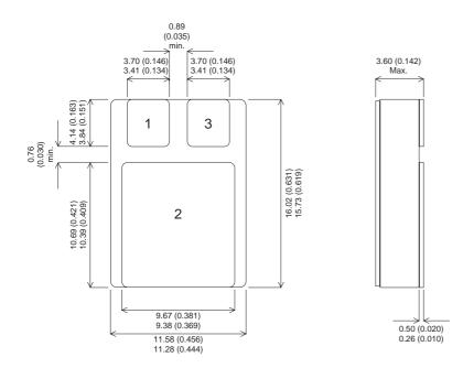
Bipolar PNP Device in a Hermetically sealed Ceramic Surface Mount Package for High Reliability Applications
